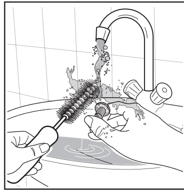
Install the valve filter back to the housing.
