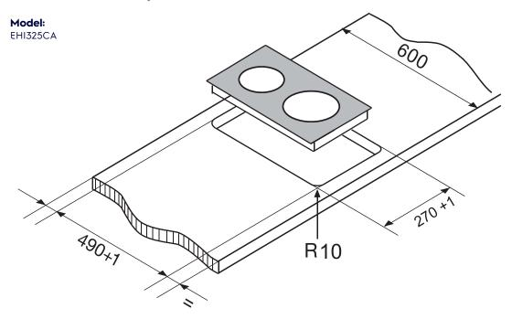
**Note:** The clearance must meet or exceed the minimum recommended for both the rangehood and cooktop. Refer to the rangehood installation manual
